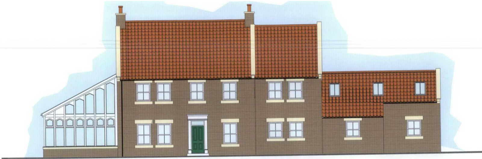
Dwelling One - Proposed South Elevation ( scale 1:100 )
